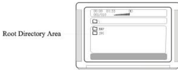
2). Press the direction button ▲▼ to move the cursor to the corresponding directory, press Play/Enter button to enter the next layer, and so on, until the desired picture is found for play.
